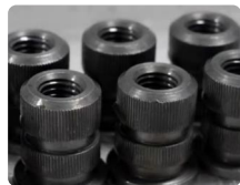
After rust removal
