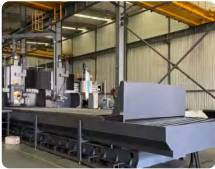
Gantry Grinding Machine
